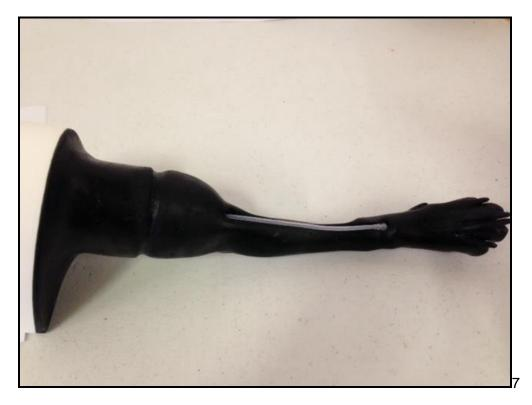
If it is ever needed, the brass tube can be replaced simply by pulling it from the top (plastic end) of the leg. The replacement brass tube can then be slid in the same way. The silicone tube held within the brass tube will extend an inch past the end of the brass and will be pushed all the way out of hole near the paw of the simulator. Once the tubing is out the bottom of the hole the clear elbow connector can be attached.
